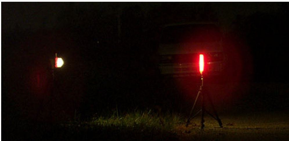
Fifty feet from a red reflector. The illuminating white light is on the left.
